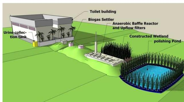
Figure 1: Schematic of school toilets connected to biogas settler and anaerobic baffled reactor at Adarsh College, in Badlapur, India (source: N. Zimmermann, 2009)<sup>1</sup>.
